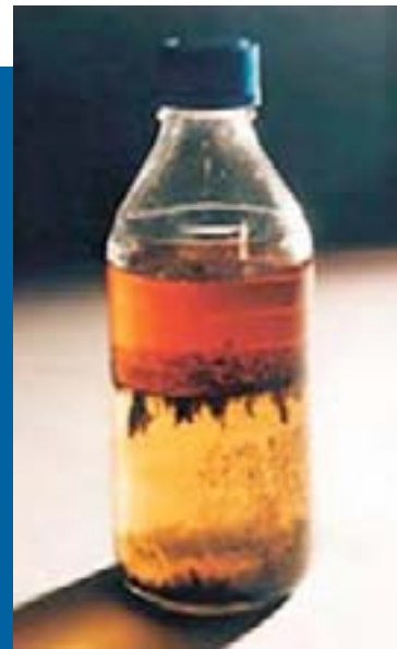
Contaminated fuel oil after being allowed to settle
